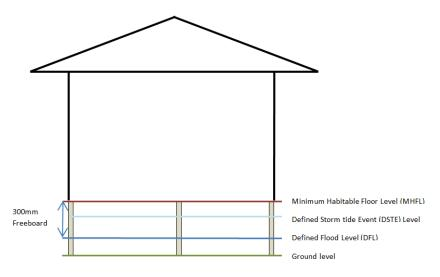
Below is an example of when the defined storm tide event (DSTE) level is higher than the defined flood level (DFL) and 300mm freeboard. The minimum habitable floor level (MHFL) can be at the same level as the defined storm tide event (DSTE) level.
