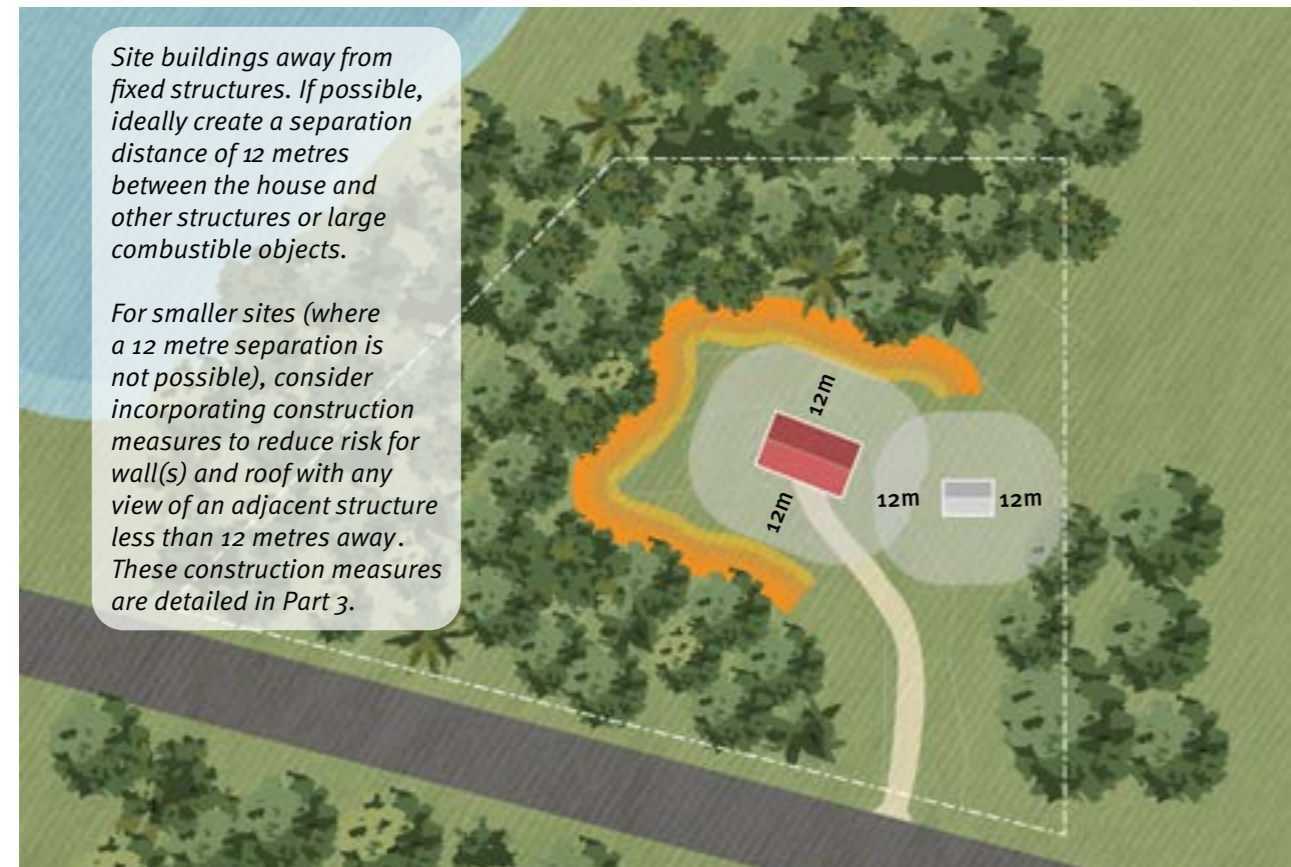
Figure 9 Siting for existing structures 19
