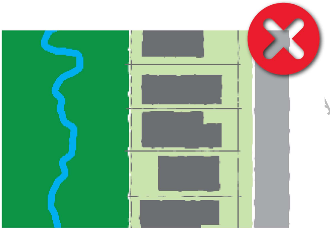
Figure 11 Lots backing directly on to waterway corridors are inconsistent with the Queensland Police Service’s guidelines on Crime Prevention Through Environmental Design (CPTED).
