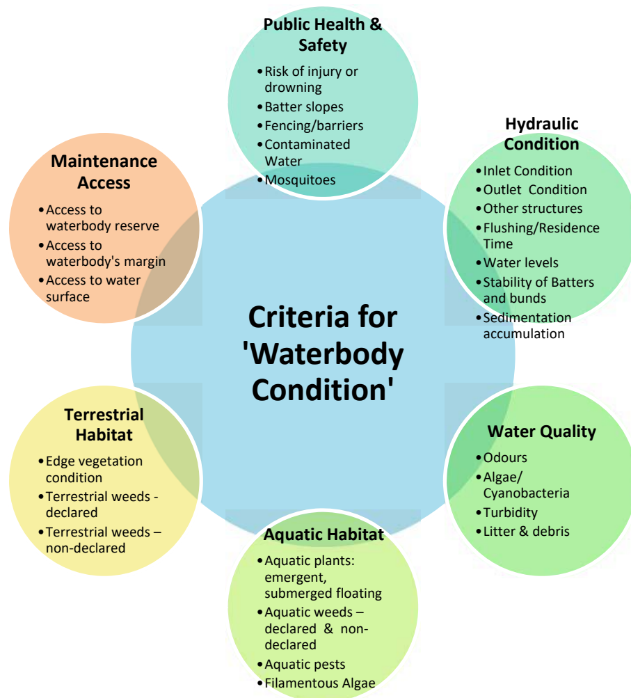
Figure 2 Condition assessment categories used to prioritise waterbodies.
